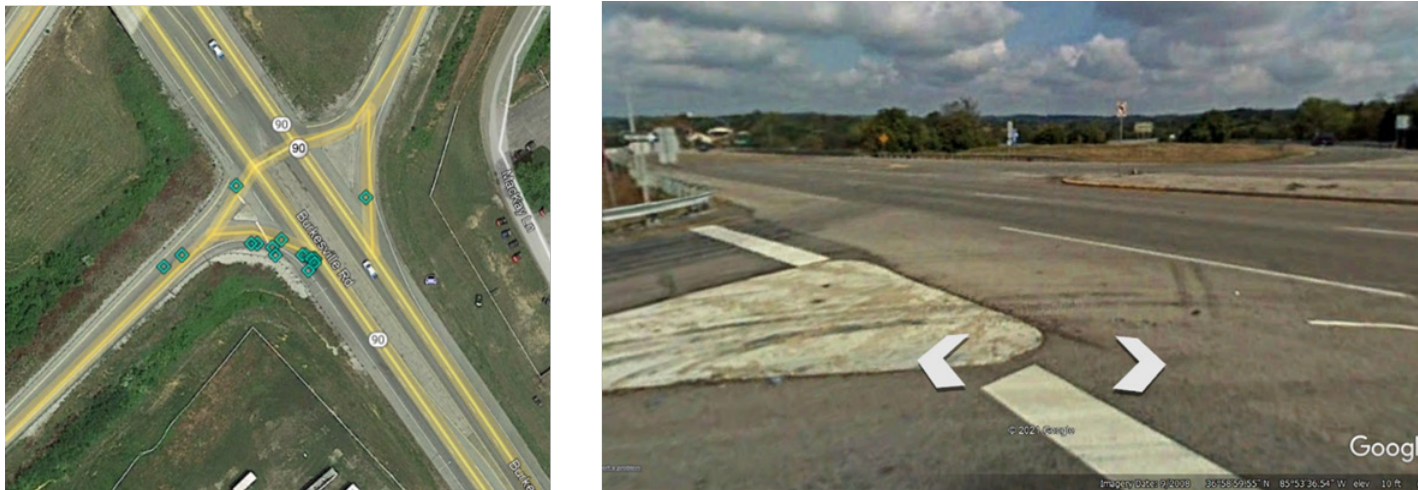
Figure 26: Exit 14 (KY 90) Eastbound Off-Ramp Crashes and Sight Distance Issues
